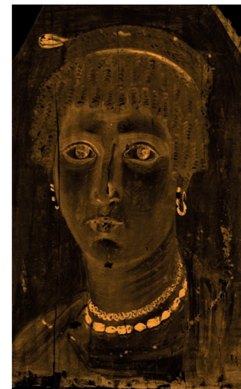
9 XRF element distribution map of iron
